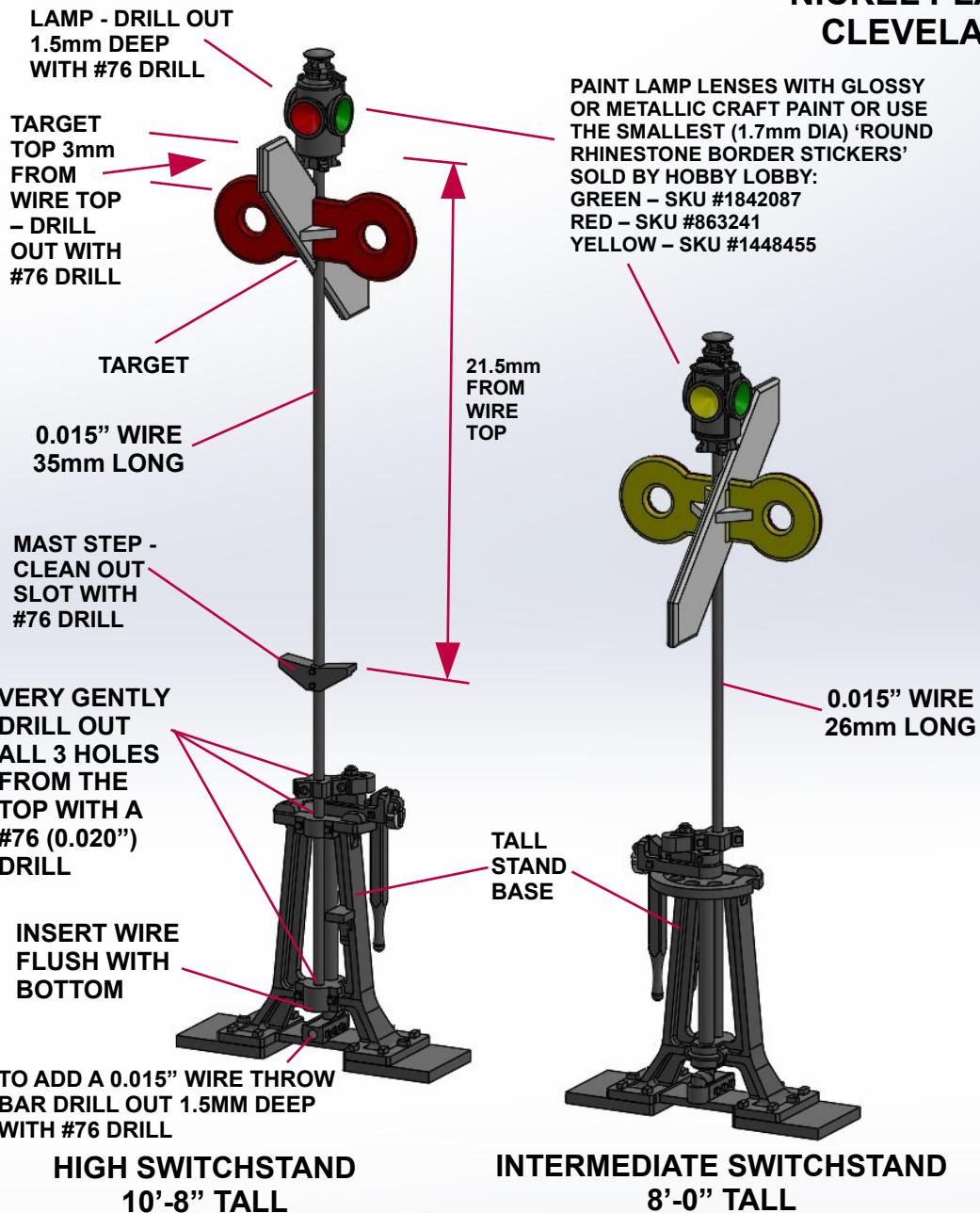
KIT INCLUDES STAND BASE, MAST STEP, TARGET, LAMP, AND 0.015" WIRE 35mm LONG.
