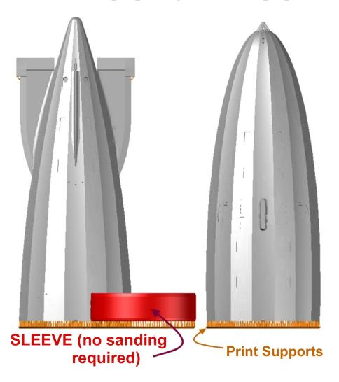
The Envelope parts arrive with the Print Supports removed however, they leave an imprint that should be removed.
