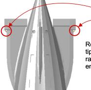
Remove these small print supports at the tip of each elevator. Use flush cutters or a razor saw and clean up with swiss files or emery paper/board.
